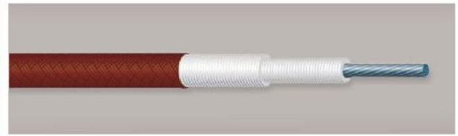
High Temperature NPC Cable Flexible nickel plated copper core. Silicone impregnated glass lappings. Silicone coated fibreglass braid.
